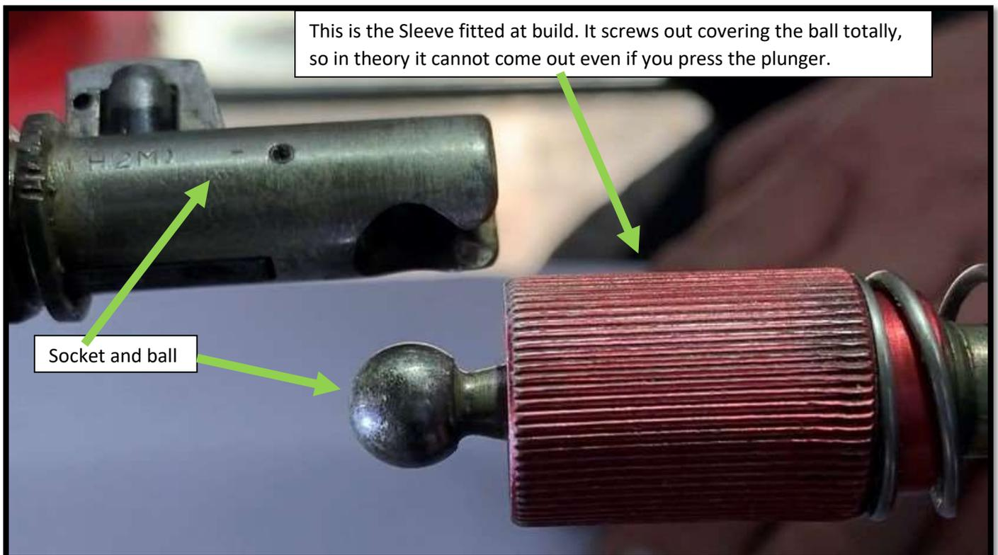
Unfortunately, some of the LS sailplanes control connections are very hard to visually inspect after the controls are connected.
