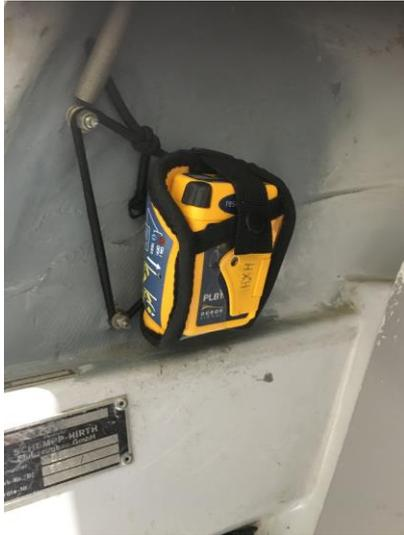
A PLB has been added to your safety equipment. It is hanging on an elastic strap on the right hand side. It can be accessed easily while you are in the cockpit should you have an emergency. Please be sure to read up on the activation procedure. A leaflet is in the side pocket.
