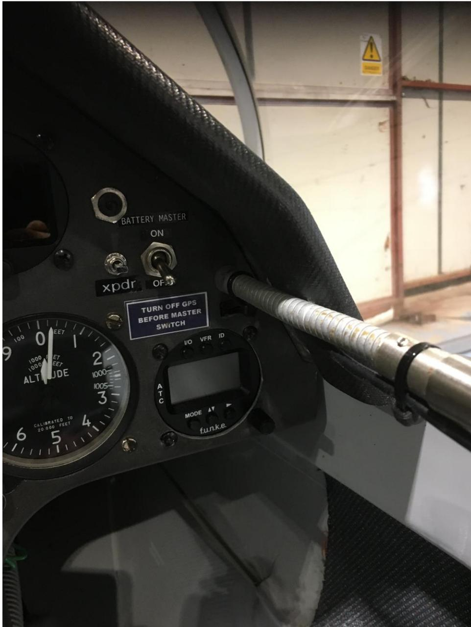
The Transponder is placed in the bottom right hand corner of the panel with a two way toggle switch left of the Master Switch. A Circuit Breaker lies immediately above the switch. This picture also shows the Oudie flexible boom mounted just above the Transponder.
