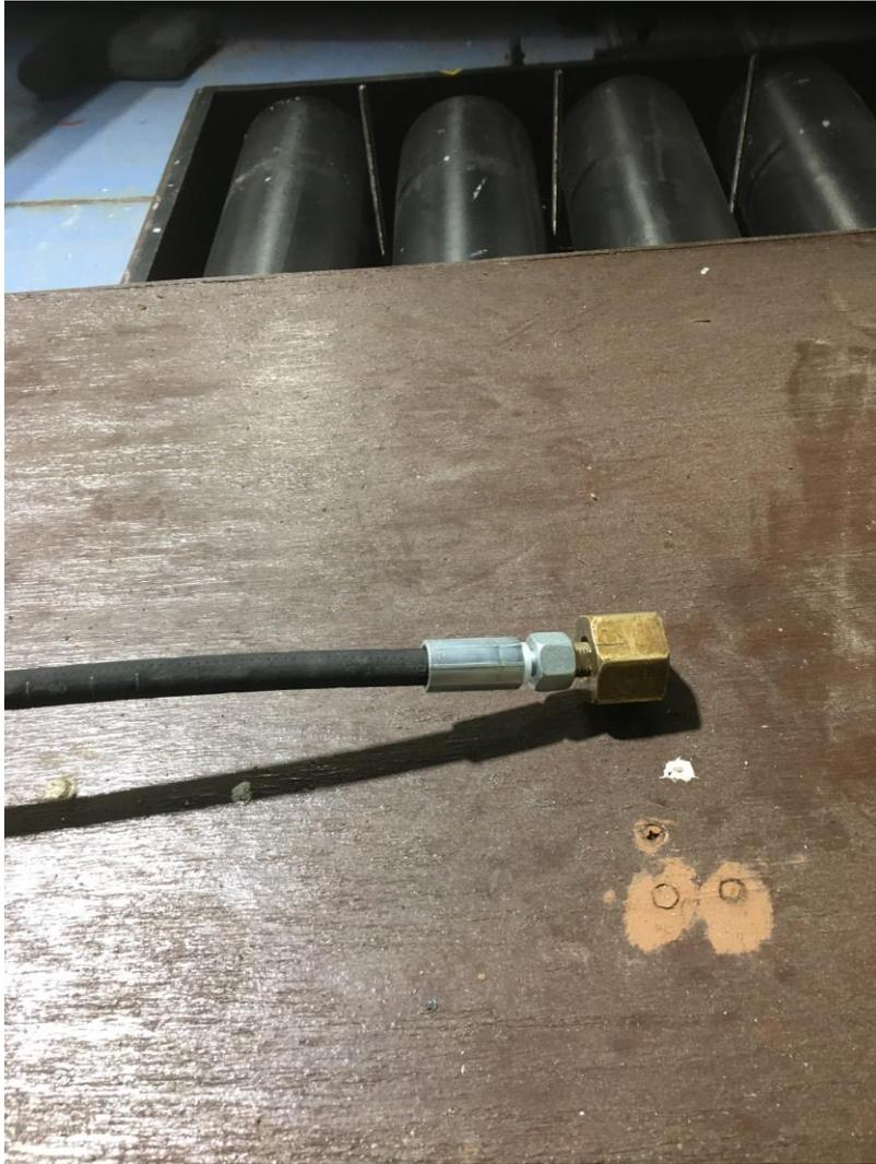
There is now an extension provided with the Oxygen fill up equipment which allows the operator to access the bottle from the cart. Just nip up the big brass nut onto the bottle valve.
