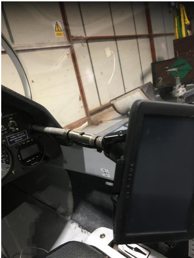
The Oudie is now mounted on a new flexible boom which brings the instrument closer to you and more easily kept clear of the control stick. The boom, like the radio mic. will provide a lot of movement but it too can only tolerate so much. There is an additional adjustment right behind the Oudie to allow you to easily rotate and adjust the instrument.
