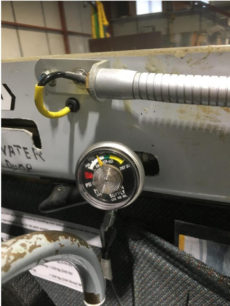
The Bottle pressure gauge is new but remains in the same position as before. You will note that the radio microphone has been replaced. Please take care not to put too severe a bend on this boom as it will break right at the fixing bracket.
