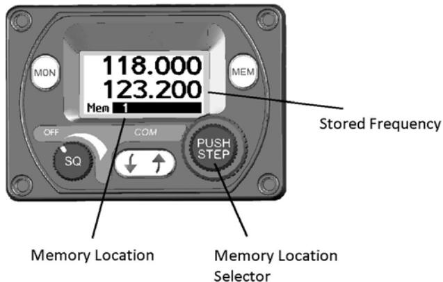
Rotating the small frequency selector knob will step through the memory locations. The standby frequency window will display the stored frequency.
