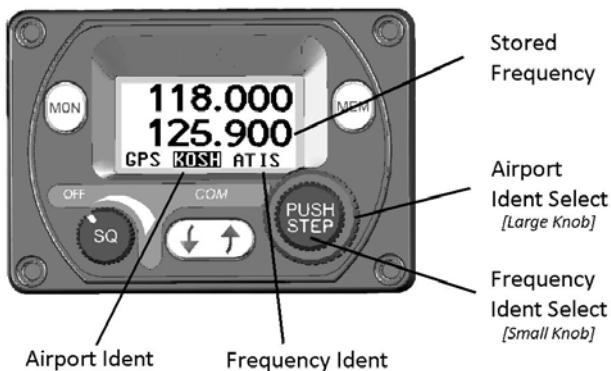
The available airports can be scrolled through using the large frequency select knob. The individual frequencies associated with that airport can be scrolled through by using the smaller frequency select knob. After you have stepped through all the loaded airports, or if there is no GPS attached, the built-in memory of the controller will be displayed.
